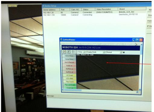
Geovision GVHTMLViewer utility allowing core Mobotix camera setting changes
